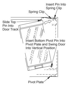
Figure 35 - Installing Optional Glass Door
